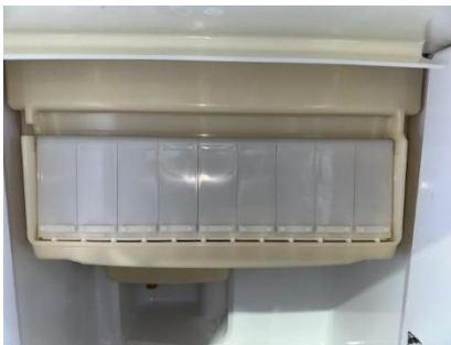
(Image of water curtain in its correct position)
